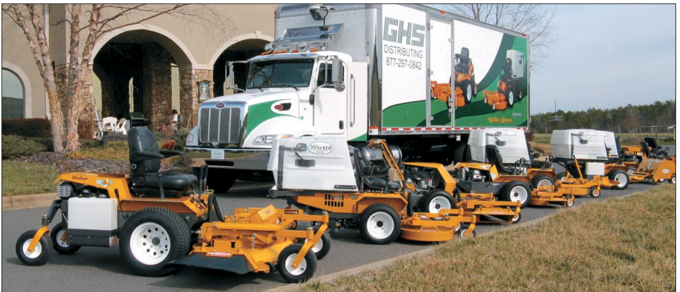
All dealer deliveries are made using this specially outfitted Peterbilt semi which can hold up to nine fully assembled Walker units and has a hydraulic "walking floor" and hydraulic tailgate for easy one-man unloading at Walker dealers, without the use of a forklift.
